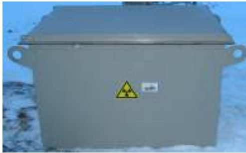
Type 5 1.5 m 3 , carbon steel, lidded Waste Box. Stored in B67 when full. For on-site use only
