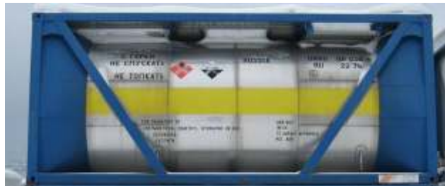
20 m 3 Toxic Waste Tanker (Heated) and mounted in an ISO Freight Container for Transportation
